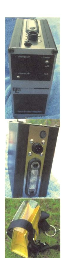
The C.M. Technology techno-light is a self contained stainless steel and extruded aluminium battery pack with a sealed 7 amp hour 12 volt gel-cell, an inbuilt battery charger, a micro-processor based lamp controller and a white led auxiliary map reading lamp. A range of suitable high powered spot-lights and xenon flood lamps are available that connect to the pack via the fused MILC locking connector.
